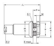
PEG Fixed socket, nut fixing, key (G) or keys (A to F, L and R), cable collet (back panel mounting)
